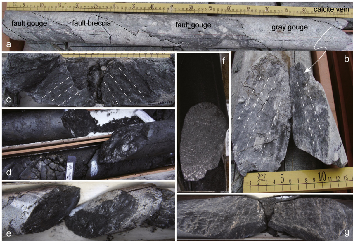
Fig. 7. Deformation structure characteristics of fault-related rocks in WFSD-1 cores. (a) Fault-related rocks at 232.50–233.33 m-depth in FZ233; (b) Steep striation in the fault plane which lies at the bottom of (a), indicating pure thrust component; (c) oblique thrust striation; (d, e, f) “Mirror structure”; (g) striation and steps in the fault plane.
