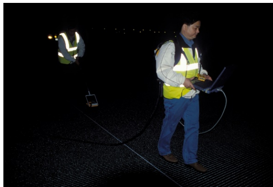
GPR survey at runway
